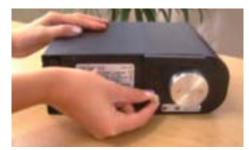
C. Rotate the locking release knob (Interlock) counter-clockwise, to the locked position. The projector may now be switched on.
