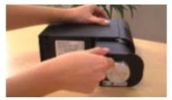
*D*. Pull the lamp cartridge handle and completely slide the lamp cartridge out of the unit.
