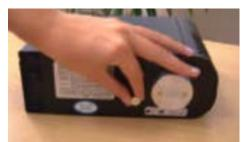
C. Rotate the locking release knob (interlock) clockwise to the open position.
