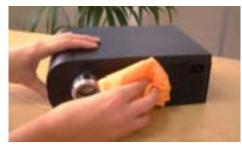
Use an air duster and cloth as follows; A. Wipe away any dust from the air inlet using the dust cloth.
